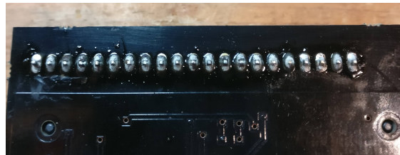
Figure 4: Soldered headers from below
