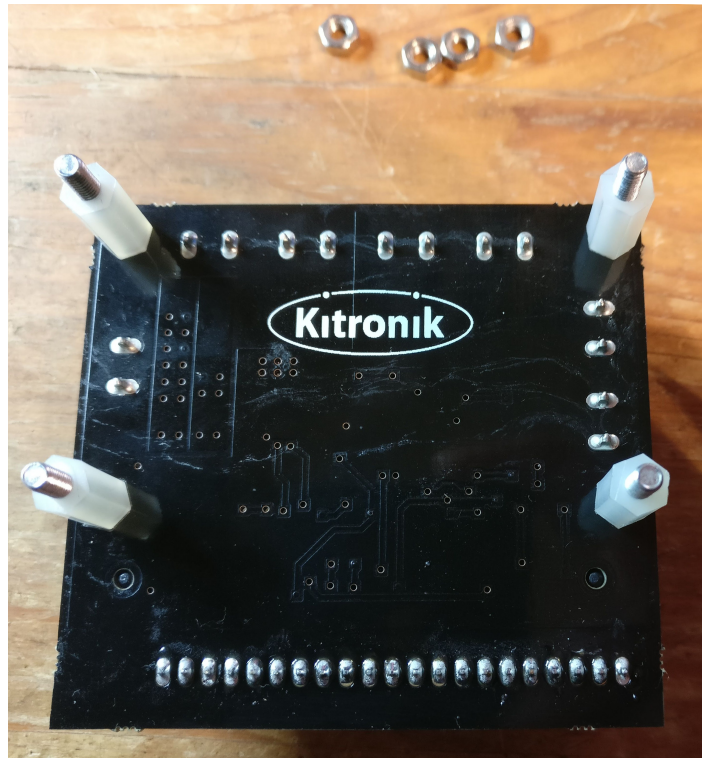
Figure 10: Motor controller with spacers
